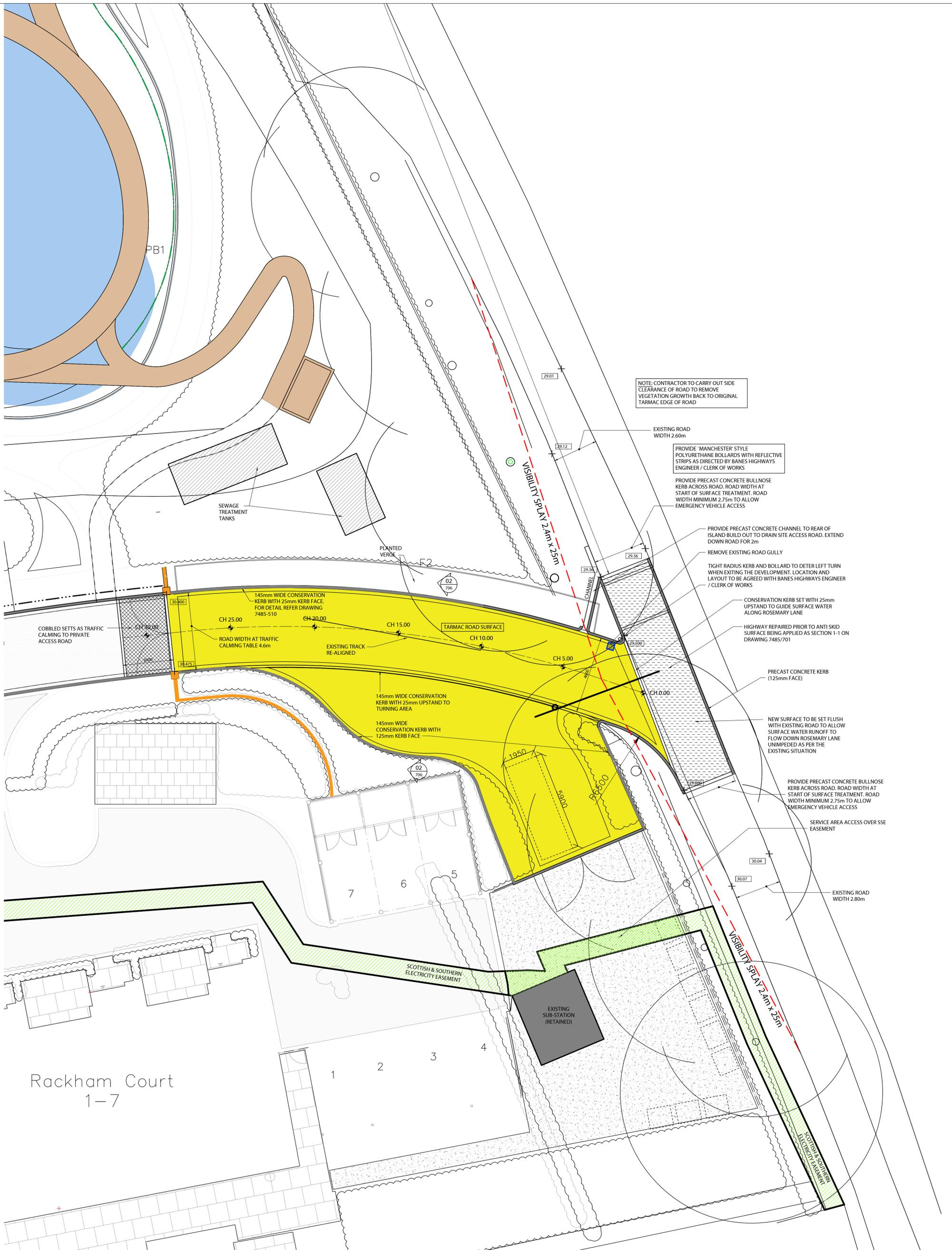
NOTE: CONTRACTOR TO CARRY OUT SIDE CLEARANCE OF ROAD TO REMOVE VEGETATION GROWTH BACK TO ORIGINAL TARMAC EDGE OF ROAD
